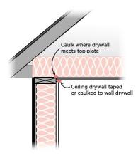
Seal the wall drywall to the top plate and ceiling drywall.
